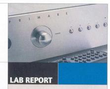
Primare's rating is 75W into 8 ohms, which seems fair – in fact, we got 81W. The increase when only one channel is driven is minimal, but into 4 ohms power very nearly doubles, and surprisingly there seems to be no dynamic headroom available, suggesting clipping is determined upstream and not at the output.
